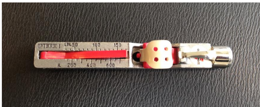
Tool for belt tension control. OPTIKRIK I. Part no. 140155.0
