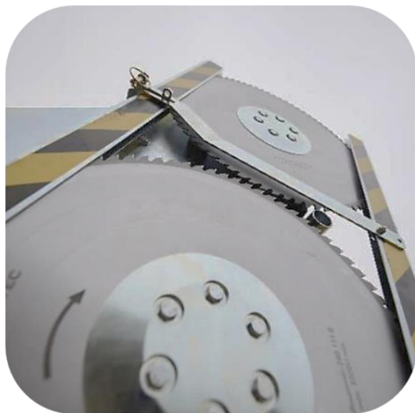
LRS Quadsaw in transport position with safety devices fitted (Protective guards for saw blades)
