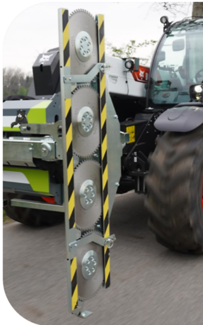
Protective guard mounted around saw blades
