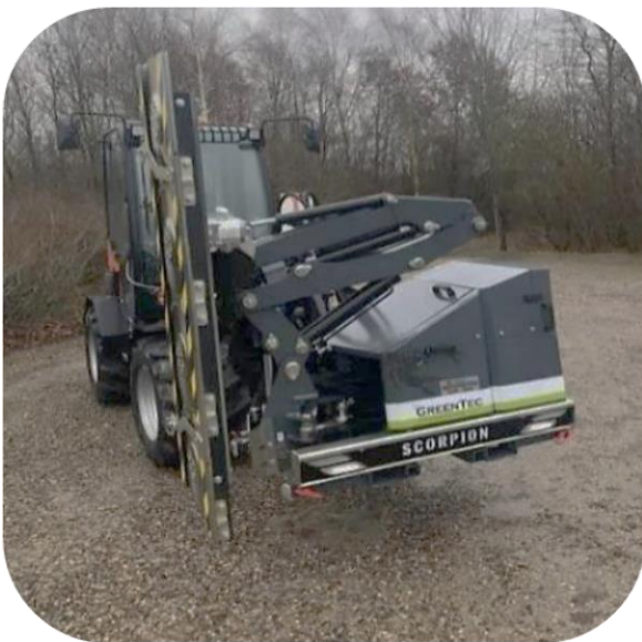
Example of transport position: LRS Quadsaw mounted together with Scorpion 3-430 boom mower. Lights free on tool carrier and vehicle
