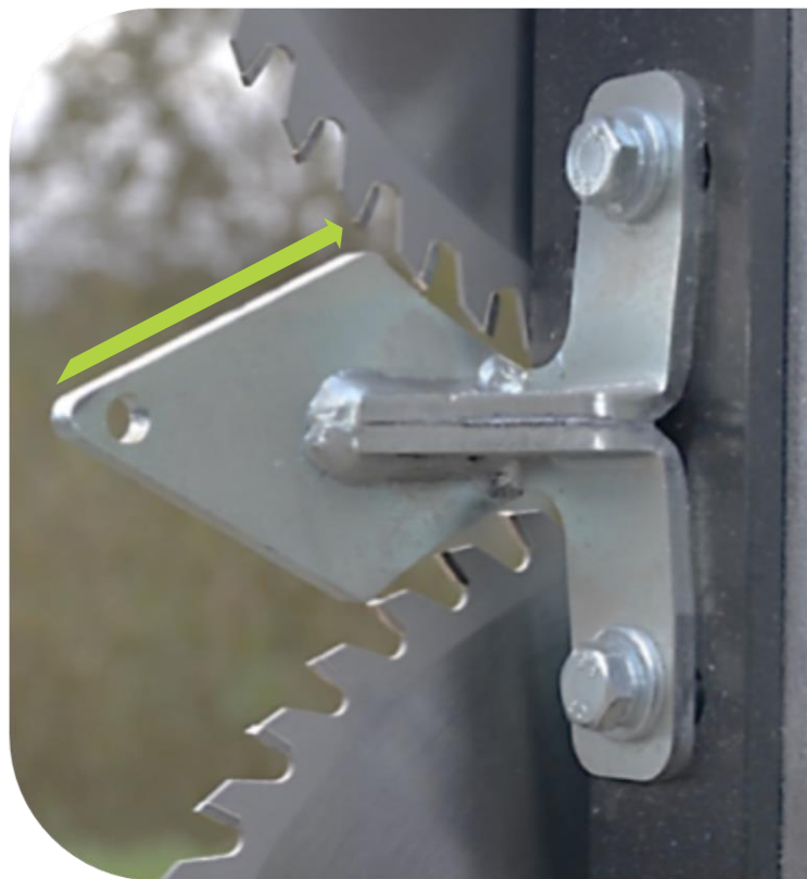
Branch guide adjusted on LRS 1602 Quadsaw
