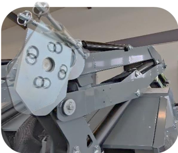
Example: Quick-release "male" adapter on Scorpion 3/4 Plus boom mower
