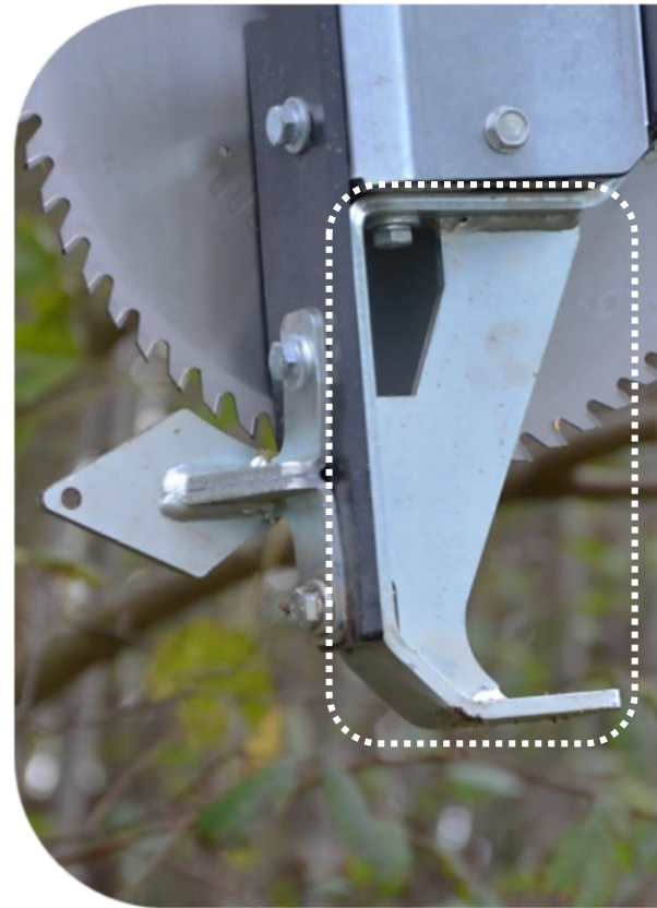
Skid shoe mounted at the lower saw blade
