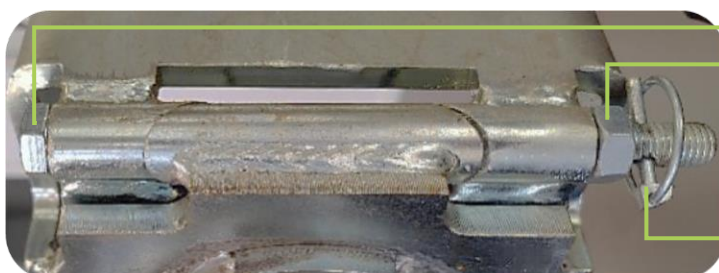
Example: Quick-release "male" adapter on Scorpion 3/4 Plus boom mower
