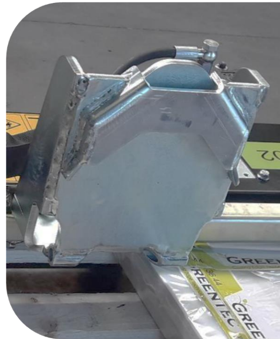
Mechanical quick-release mounted on LRS 1602 Quadsaw: ("female" part)
