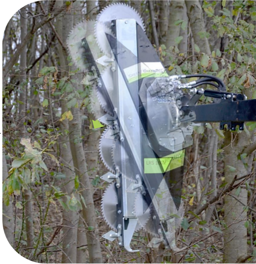
Setting the cutting angle on the LRS 1602 Quadsaw, mounted on a PUMA 2803 Multi Carrier
