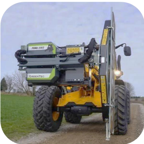
Example of transport position: LRS 2002 Quadsaw mounted together with Scorpion 3-430 boom mower. Lights free on tool carrier and vehicle
