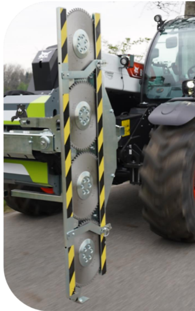
Protective guards mounted around saw blades
