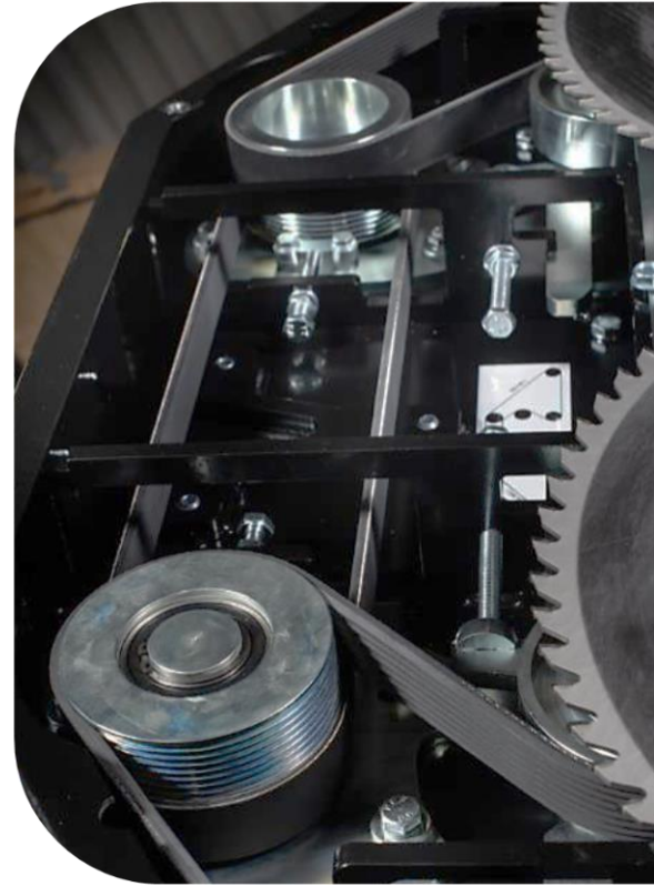
Power-band belt drive on LRS 2402 Quadsaw
