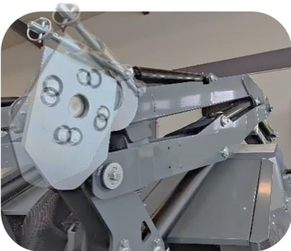
Example: Quick-release "male" adapter on Scorpion boom mower.
