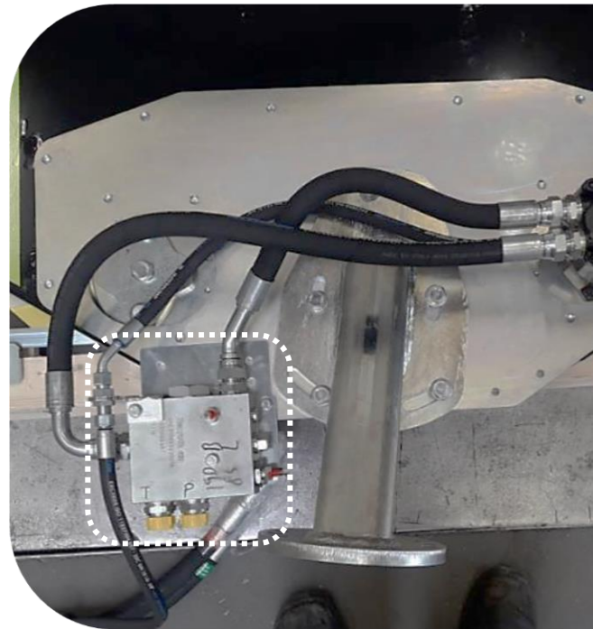
Oil flow divider (universal) on LRS 2402 Quadsaw
