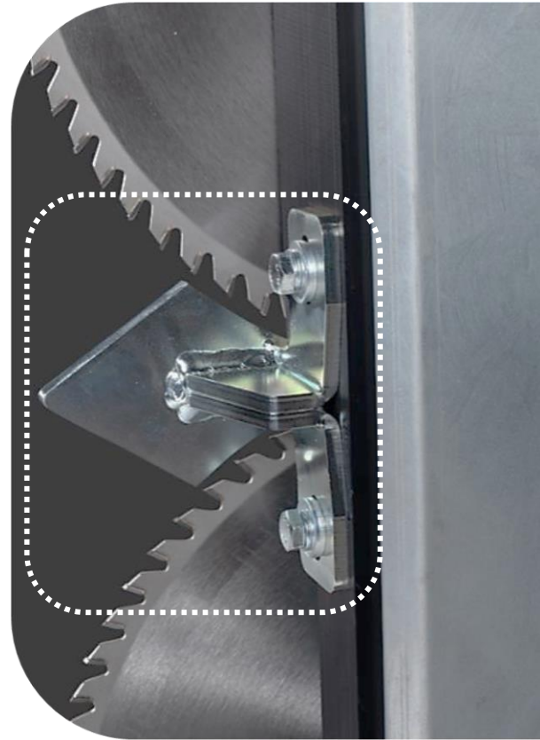
Branch guides at each saw blade
