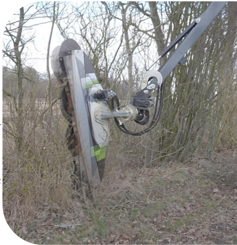
Setting the cutting angle on the LRS 2402 Quadsaw
