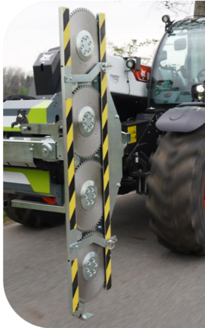
Protective guards mounted around saw blades
