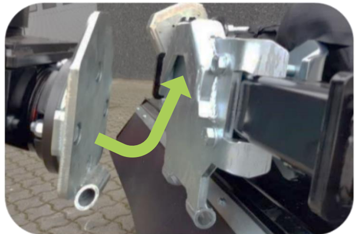
Example: Quick-release "male" adapter on boom mower is paired with the "female" adapter on the attachment tool.
