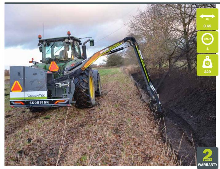
The Rotary Ditch Cleaner GR 70 is a highly efficient machine for cleaning of smaller ditches and streams. The sludge and weeds are effectively removed and thrown up on the cliff.
