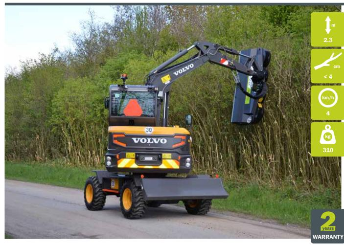
The Rotary Mulcher RM 232 provides enormous capacity and perfect performance. In one operation, branches are cut and instantly mulched.
