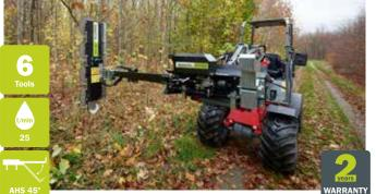
The Multi Carrier HXF 2302 can easily be mounted on smaller vehicles, such as skid steer loaders and compact tractors with a minimum weight of 1,200 kg (2,646 lb).
