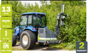
The Scorpion 4 series consists of compact reach mowers intended for smaller tractors, implement carrier, skid steer loaders and the like. The models are available in horizontal working widths of 3.3 and 4.3 m (10'10" and 14'1").
