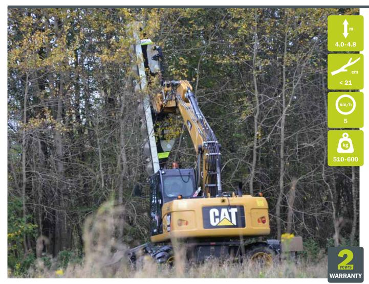
GreenTec presents the world's largest saw with working widths of 4.0 and 4.8 m for municipal and farming use. The saw is fitted to large diggers, excavators and loaders. It goes without saying that the capacity is enormous.
