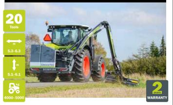
The Scorpion 6 series is available in four models and is designed for medium-sized tractors with a weight of at least 4,000 kg (8,818 lb).
