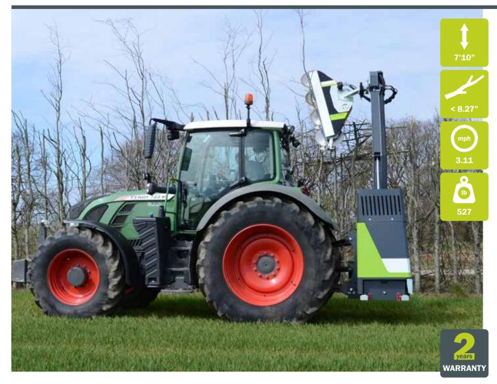
The Quadsaw LRS 2402 is the second largest saw in the series and has an enormous power and capacity. Branches up to 8.27" are cleanly cut - experienced drivers can manage branches up to 15".
