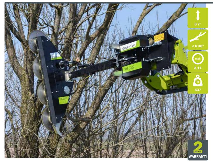
The Quadsaw LRS 2002 has an unmatched capacity with its four saw blades and low maintenance costs. The quadsaw is produced in high-strength steel with a low weight of 437 lb. All branches receive a smooth and clean cut.
