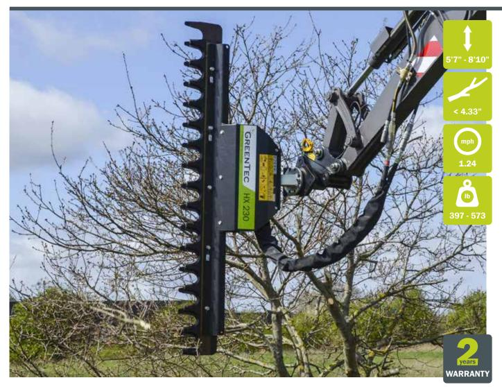
A very strong and effective cutterbar used for cutting back trees and bushes. It has a clean cut and does not leave split or frayed branches. The cutterbar can be attached to reach mowers, excavators and the Multi Carrier HXF 3302.
