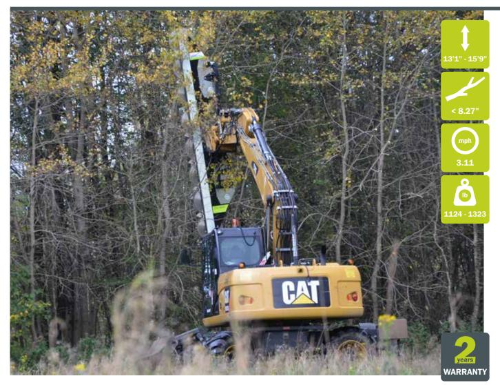
GreenTec presents the world's largest saw with working widths of 13'1" and 15'9" for municipal and farming use. The saw is fitted to large diggers, excavators and loaders. It goes without saying that the capacity is enormous.
