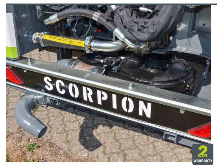
The Leaf Blower LG is a high-pressure blower that is hydraulically driven through the tractor's hydraulics.
