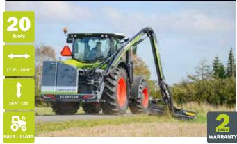
The Scorpion 6 series is available in four models and is designed for medium-sized tractors with a weight of at least 8,818 lb.
