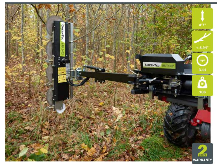
The Quadsaw LRS 1402 is a small yet powerful quadsaw with four saw blades and a working width of 4'7".
