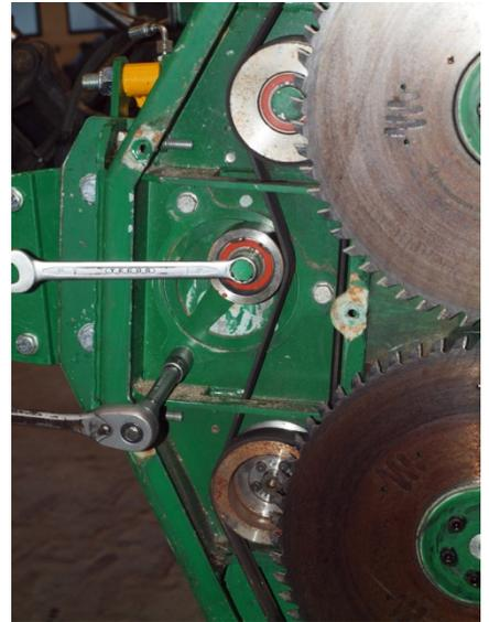
Check torque on the center belt
