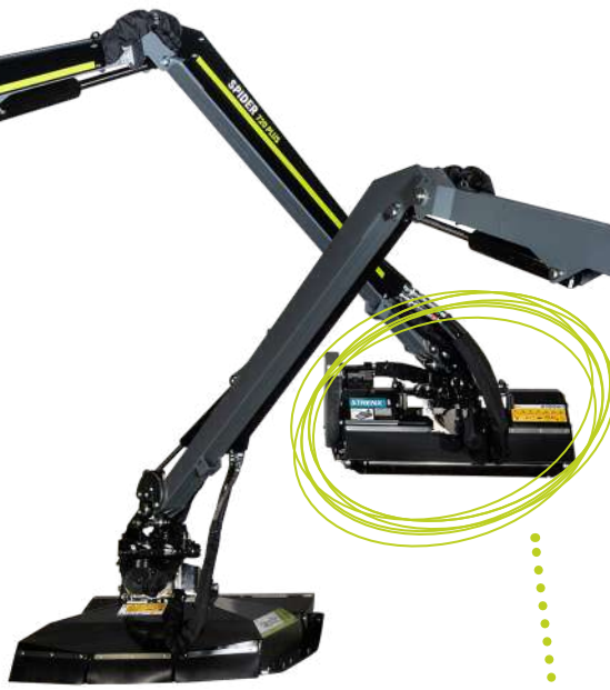
The arm is controlled from the cabin and can be moved from the right to left side and into the driver's field of vision.
