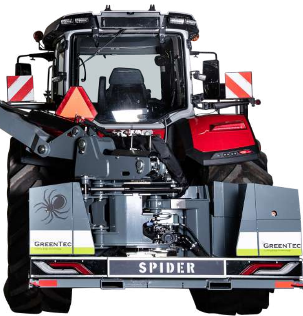
The arm is controlled from the cabin and can be moved from the right to left side and into the driver's field of vision.
