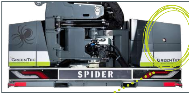
The 220 liter hydraulic tank is located on the right side, and the hydraulic valves and oil cooler are located on the left side.
