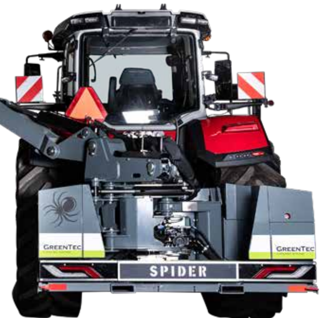
The arm is controlled from the cabin and can be moved from the right to left side and into the driver's field of vision.
