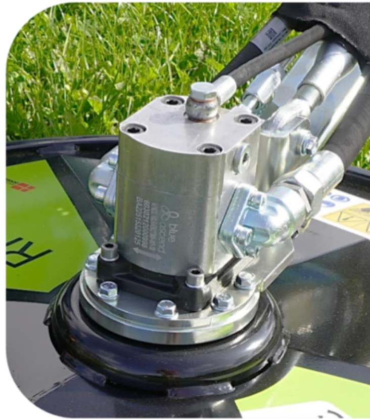
Hydraulic gear motor
