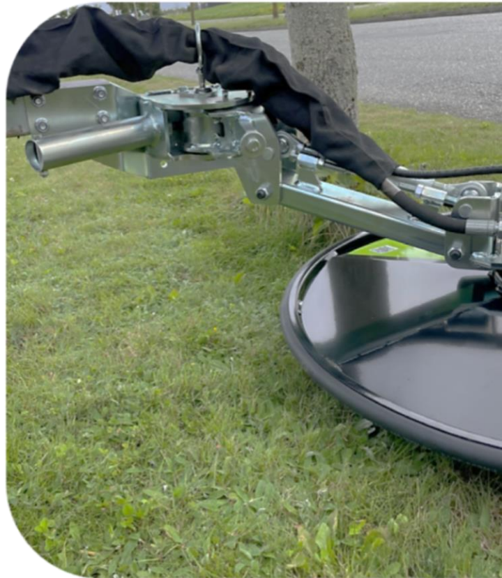
Spring-loaded arm system / "break-back" function
