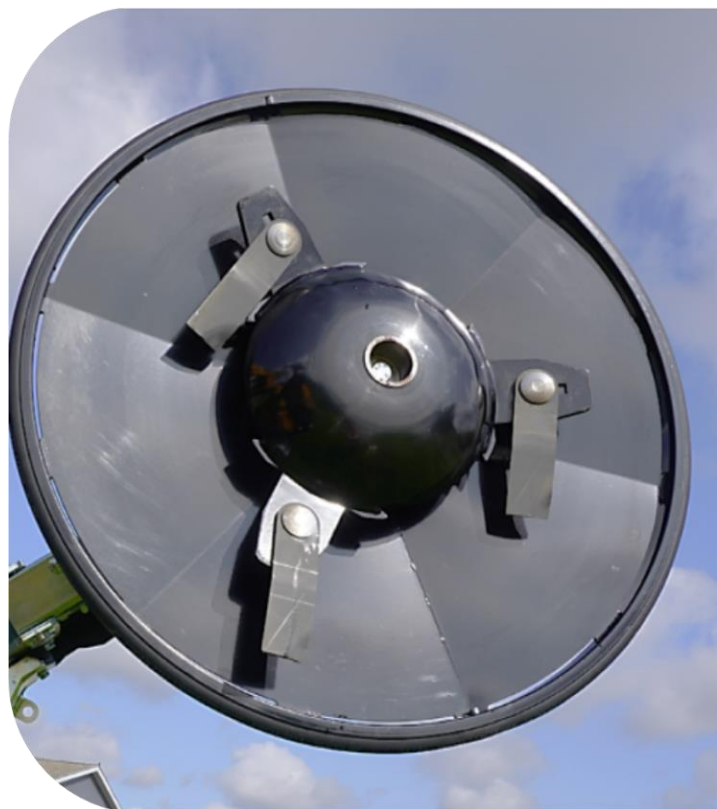
Blade rotor with hardened steel blades
