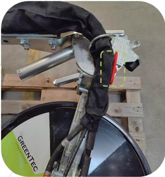
RI Barrier Mower in retracted and locked position (Transport position)
