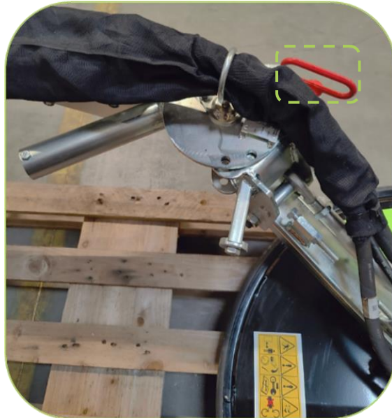
RI Barrier Mower in extended and unlocked position (Working position)
