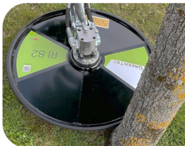
Rubber protection around cutting head
