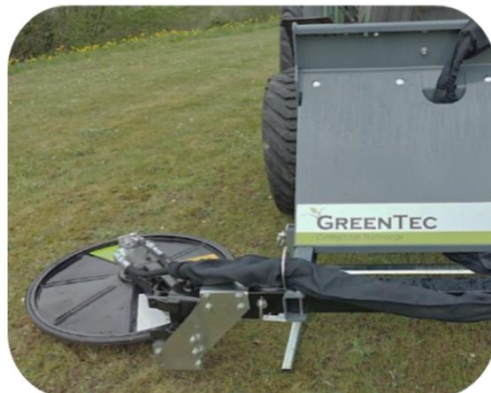
FOX Multi Carrier mounted with RI Barrier Mower in working position. The attachment tool can be further extended in reach using the Multi Carrier's arm system.
