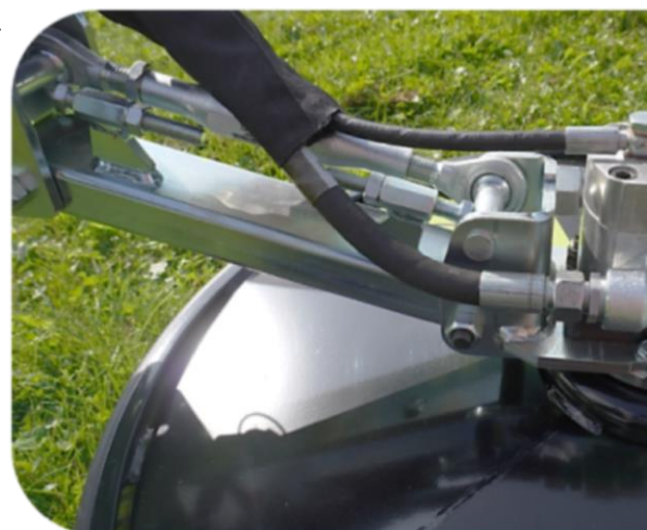
Adjustable suspension on RI Barrier Mower
