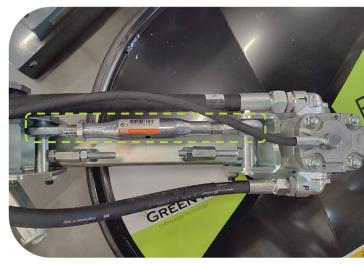
Position of the top-link for adjusting the working height of the suspension
