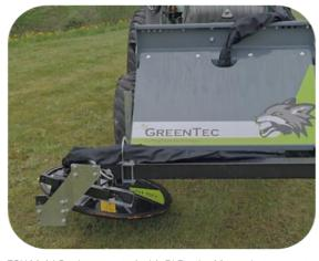
FOX Multi Carrier mounted with RI Barrier Mower in transport position. The attachment tool is turned inwards towards the vehicle, for maximum traffic safety.
