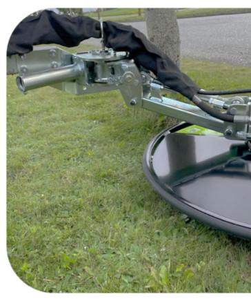
Spring-loaded arm system / "break-back" function
