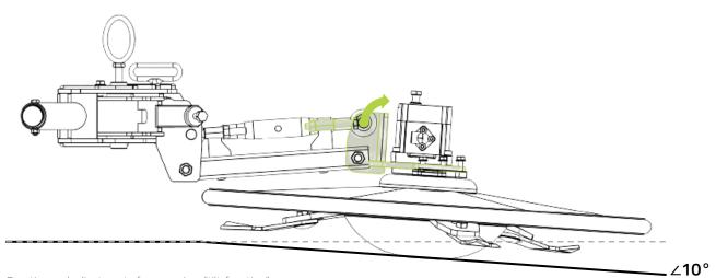
Function and adjustment of suspension: "tilt-function"
