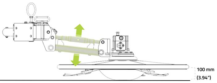
Function and adjustment of suspension: working height
