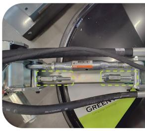
Position of screws for adjusting the "tilt"-function
