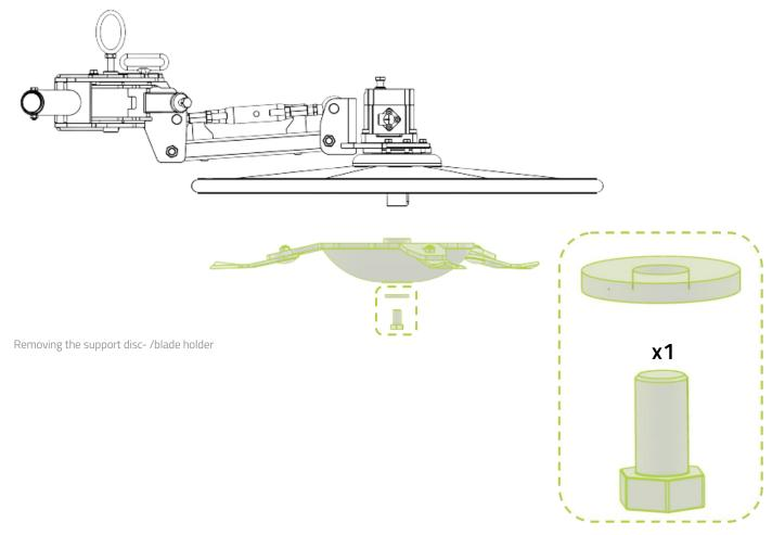
2. With the support disc-/blade holder detached from the cutting head, loosen and remove all 3x blade bolts (M12 x 1.5) at the blades:
