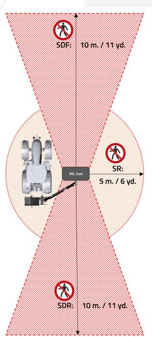
Figure 5 – Safety zones (Vehicle/attachment tool)
