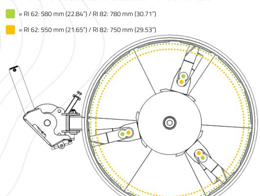
1. Support disc-/blade holder on the underside of the RI Barrier Mower's cutting head is removed using a set screw (M16 x 25) and a washer:
