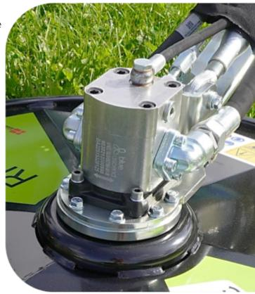
Hydraulic gear motor
