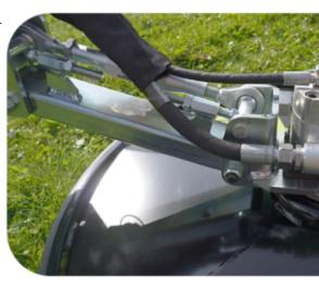
Adjustable suspension on RI Barrier Mower
