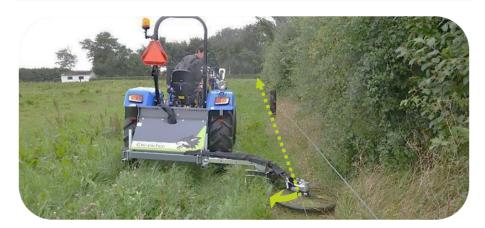
The forward speed when using the RI Barrier Mower must be max. 3-4 km/h (1.86-2.49 mph) and must always be adjusted so that the cutting result is optimal.
