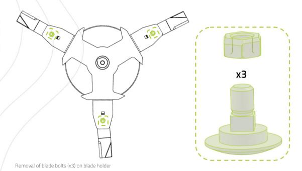
3. The blades are moved to either the inner/outer hole on each blade holder.
