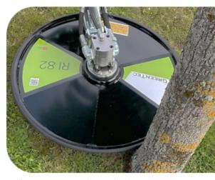
Rubber protection around cutting head
