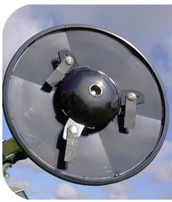
Blade rotor with hardened steel blades
