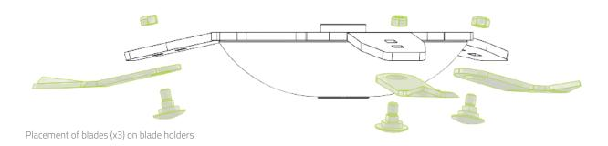
4. With the blades attached to the knife holders, the support plate on the underside of the RI Barrier Mower's cutting head can be mounted again using the set screw and washer. The set screw (M16 x 25) is then tightened with: 197 Nm (145.30 lbf·ft)
