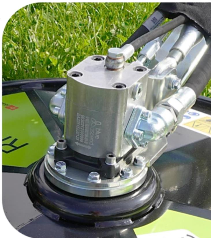
Hydraulic gear motor
