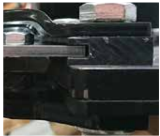
PLASTIC GUIDING OF THE CUTTER BAR
