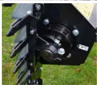
HD PLANETARY GEARBOX WITH CAST IRON ENGINE
