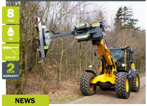
Puma 3303 is the largest model in the series and is mounted on telehandlers, large front loaders and excavators. As standard, all Pumas have automatic hydraulic security with pre-pressure. This means that you can maintain a constant driving speed. When encountering a large branch, the arm retreats slightly and then moves forward again when the branch has been cut. A large range of tools is offered for every task when it comes to tree maintenance.
