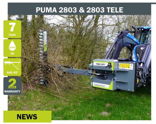
Puma 2803 is mounted in a few minutes on front loaders or large skid steer loaders. A huge selection of tools makes hedge and tree trimming a breeze. The Puma can also be fitted with the Barrier Mower RI 82, whereby grass mowing is also possible. Puma 2803 requires 40 l/min oil supply - in return you get an unrivaled capacity, regardless of which tool is chosen. An electric remote control is offered as optional equipment.
