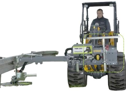
RI 82 Barrier Mower on a PUMA 2303 Multi Carrier: Support feet/stands up-raised.
