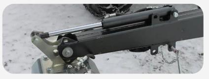
For electro-hydraulic adjustment (Plus models) an electrically controlled valve block incl. a cylinder is used for adjusting the cutting angle of the attachment tool. The cylinder is adjusted using the supplied remote control.
