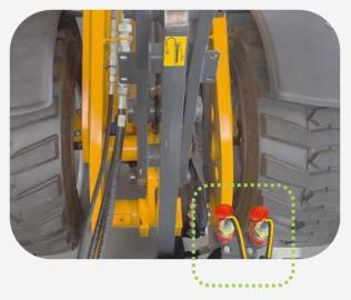
For PUMA 2303 Plus-models with e-control: a power cable from the transmitter/oil flow divider is connected with a 3-pin 12V connector, onto the vehicle's 12V-socket. \*
