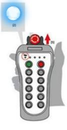
3. Press: 🕐 to connect the remote control to the receiver on the PUMA 2303 Multi Carrier.
