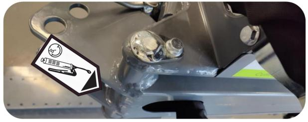
Location of the grease nipple at the inner side of the Multi Carrier swing arm
