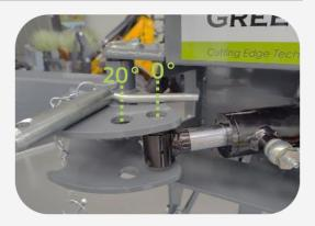
\* It is recommended to use the 20°-degree angle when using the PUMA 2303 Multi Carrier with either RI-82 Barrier Mower and/or BR 70 Weed Clearing Brush. For any other approved attachment tool, the 0°-degree angle is recommended!
