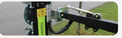
With hydraulic adjustment (optional equipment), a cylinder is used to adjust the cutting angle of the attachment tool. The cylinder is adjusted directly from the vehicle's hydraulic system from the driver's seat. \*
