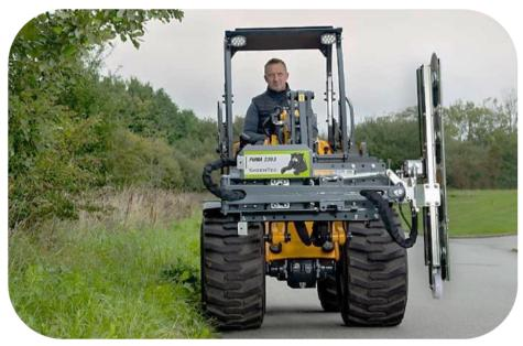
Example of transport position: Lights free on the vehicle, clear view, with safety devices **5.6.3** on the attachment tool facing the vehicle for maximum traffic safety.
