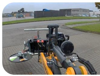
Example PUMA 2303 Multi Carrier mounted on a front-loader w/ RI 82 Barrier Mower
