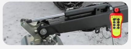
\* The hydraulic cutting angle adjustment requires an additional 1 x DA-outlet from the vehicle. From here, the angle of the attachment tool is adjusted directly from the vehicle's own hydraulic controls. Always refer to the user manual of the vehicle!
