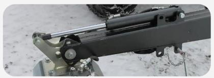
For electro-hydraulic adjustment (Plus models) an electrically controlled valve block incl. a cylinder is used for adjusting the cutting angle of the attachment tool. The cylinder is adjusted using the supplied remote control.
