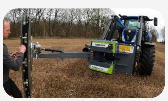
The safety pin is mounted again between the swing arm and impact cylinder, in one of the 2 settings: 0° or 20° working angle.
