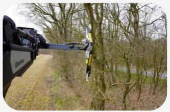
The forward speed when using the attachment tool must be max. 5-7 km/h (3-4mph) but must always be adjusted so that the cutting result is optimal.
