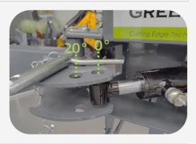
\* It is recommended to use the 20°-degree angle when using the PUMA 2803 Multi Carrier with either RI-82 Barrier Mower and/or BR 70 Weed Clearing Brush. For any other approved attachment tool, the 0°-degree angle is recommended!
