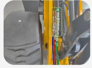
DK:TRYK UK:PRESSURE D:DRÜCK The Multi Carrier must be supplied with minimum 40 I/min @ 180 bar (10.57 gpm @ 2610 psi) from the vehicle's hydraulic outlets.
