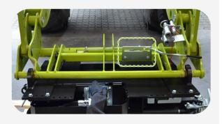
4. Carefully begin to lift the PUMA 2803 Multi Carrier into its working position. Transport brackets fitted upon delivery are removed and replaced with the correct support legs (3 pcs.). These are included in the box with screws etc.
