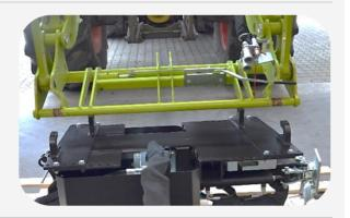
Make sure that the hooks from of the loader bracket have a firm grip on the front loader frame and make sure that holes and locking pins are flush, before locking the front loader locking mechanism to secure the Multi Carrier onto the loader frame. The PUMA 2803 Multi Carrier is now mechanically mounted.
