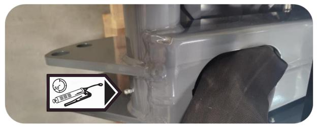
Location of the grease nipple at the inner side of the PUMA 2803 Multi Carrier swing arm
