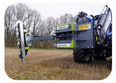
PUMA 2803 Multi Carrier with LRS 1402 Quadsaw In vertical position
