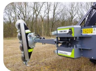
Example of PUMA 2803 Multi Carrier mounted on a front-loader w/LRS 1602 Quadsaw.
