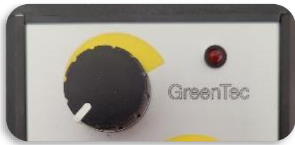
AHC-potentiometer op bedieningspaneel in positie "0"
