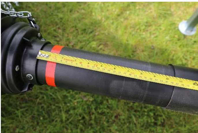
Figure 6 - Input PTO Minimum Free Travel – 260mm
