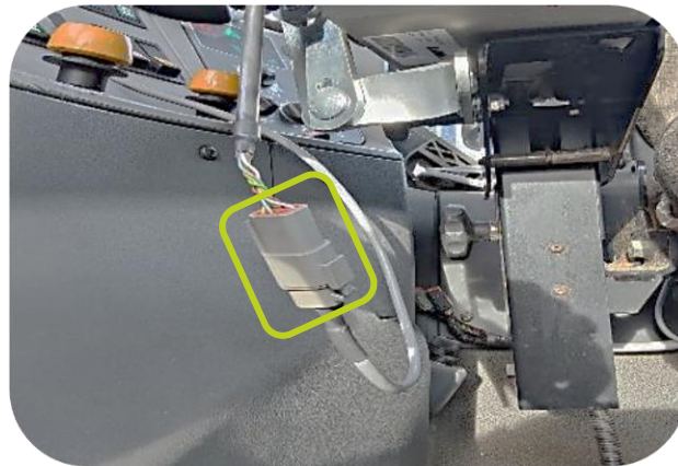
Connection of joystick using 1 plug/cable from control panel
