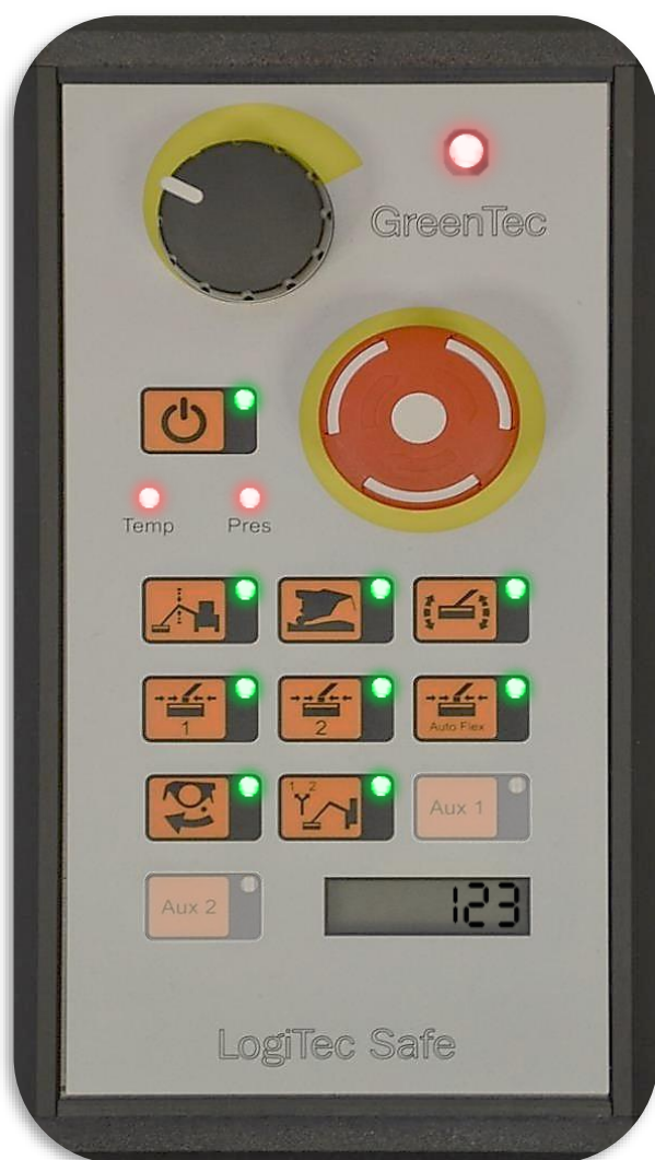
LogiTec Safe control panel on the Scorpion 490 boom mower
