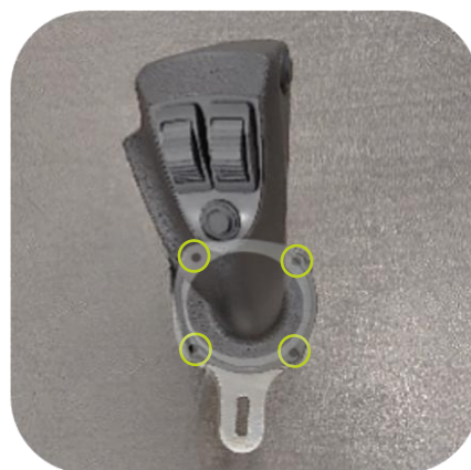
Attaching the mounting bracket (part 1) to the underside of the joystick
