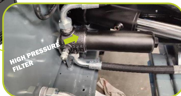
High pressure filter on Scorpion 490 boom mower
