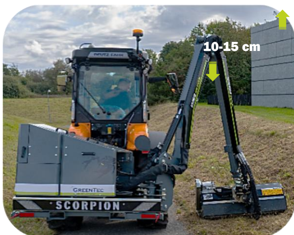
Driving with hydraulic float-function (arm) on Scorpion 490 boom mower
