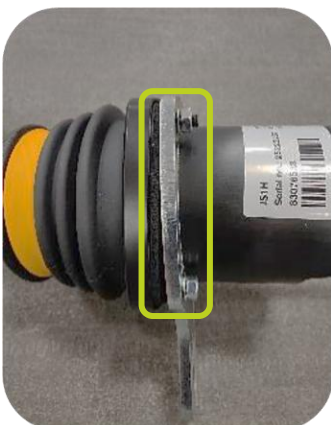
Attaching the mounting bracket (part 1) to the underside of the joystick
