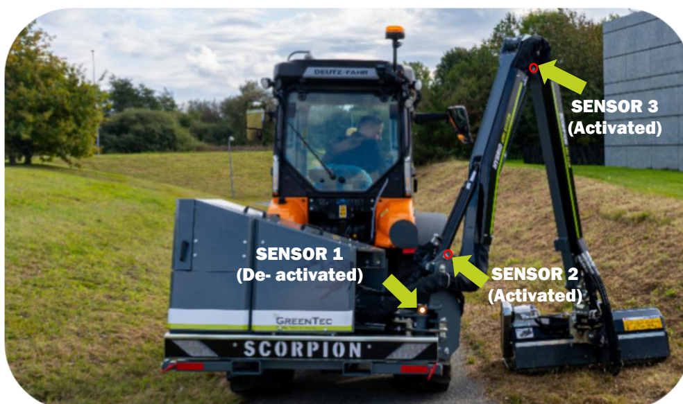
2 out of 3 safety sensors blocked and thus activated: Scorpion 490 boom mower
