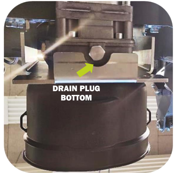
Drain plug for gearbox on Scorpion 490 boom mower
