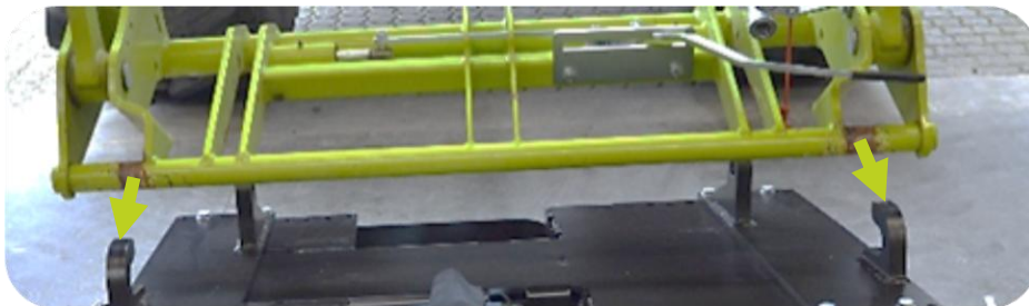
Example of vehicle lift system fitment with loader bracket / special adapter
