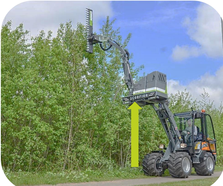
Scorpion 490 arm mower elevated using front loader with mounted HS 172 hedge trimmer
