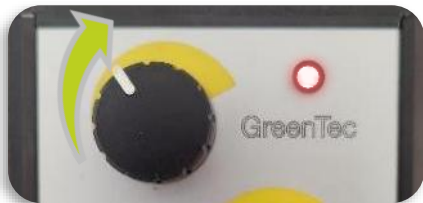
AHC potentiometer on control panel: enabled and adjusted
