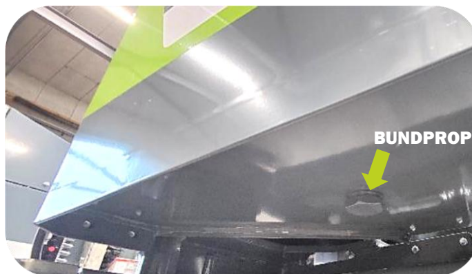
Drain plug for oil tank on Scorpion 5-830 boom mower
