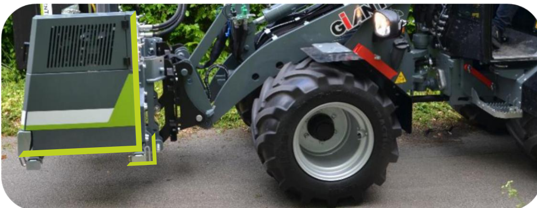
Scorpion Basic lifted and mounted using neck mount on vehicle lift system in vertical position
