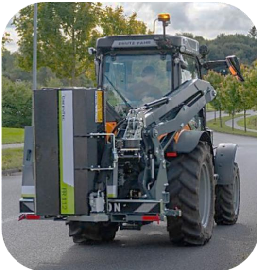
Example of transport position: Scorpion 490 boom mower and FR Flail mower (rear mounted): All lights free on the mower and vehicle
