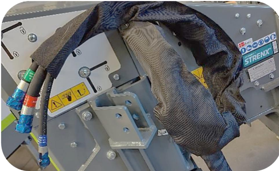
Hydraulic hoses from Scorpion 490 Basic boom mower to the vehicle
