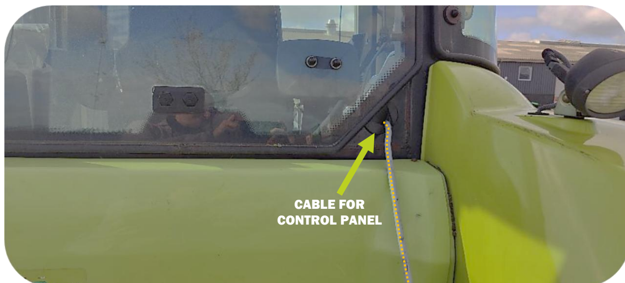
Routing of the cable from the boom mower to the cabin of the vehicle
