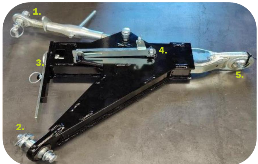
4-point linkage system Scorpion 490 boom mower
