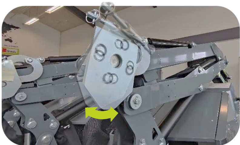
Mechanical quick coupling for attachment tools on a Scorpion Standard
