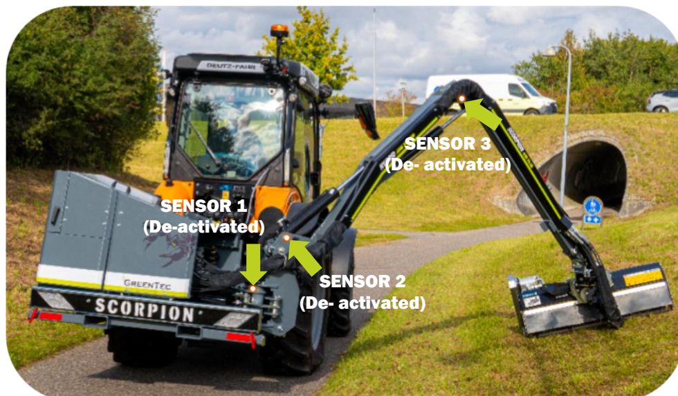
All safety sensors free, and deactivated: Scorpion 490 boom mower
