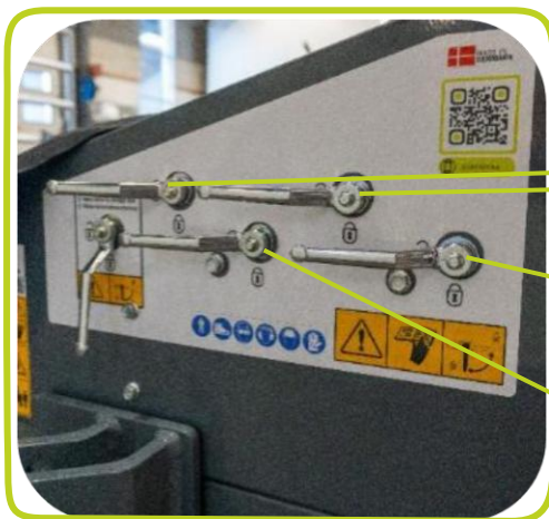
Stop valves (4 pcs.) for cylinder locking/transport position, plus 1 for attachment tool change
