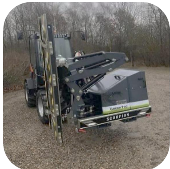
Example of transport position: Scorpion 490 boom mower and LRS Grensav (front mounted): Safety shielding mounted on saw blades
