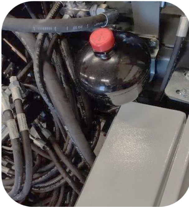
Accumulator (32 bar) on the Scorpion 490 boom mower
