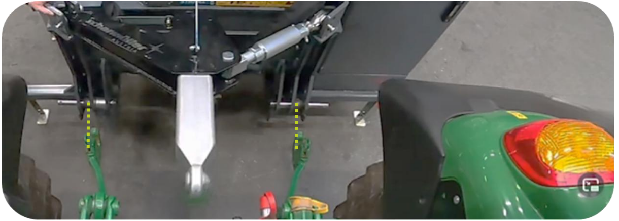
Carefully back the vehicle up to the mounting points on the Scorpion 490 boom mower
