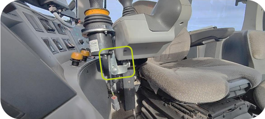
Joystick with angled mounting brackets, bolted onto vehicle console/armrest
