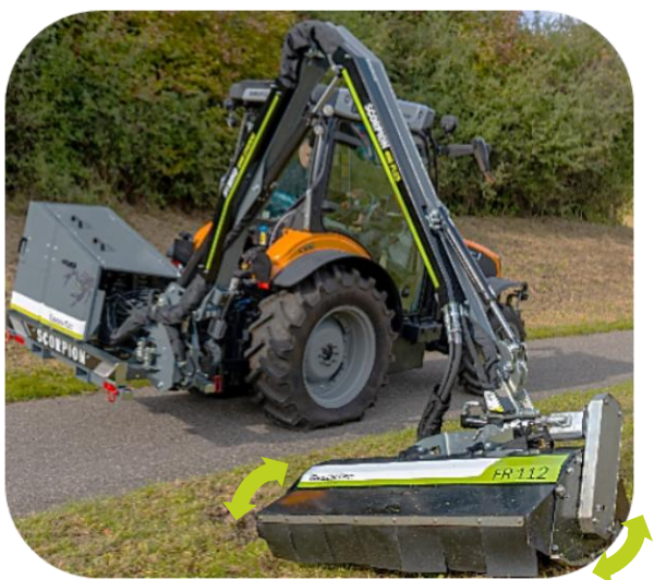
Driving with hydraulic float-function (att. tool) on Scorpion 490 boom mower
