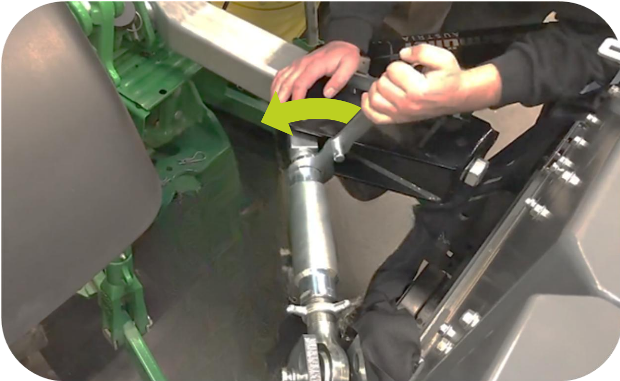
Adjustment of transverse top draw bar for tensioning of the stabilization between vehicle and boom mower
