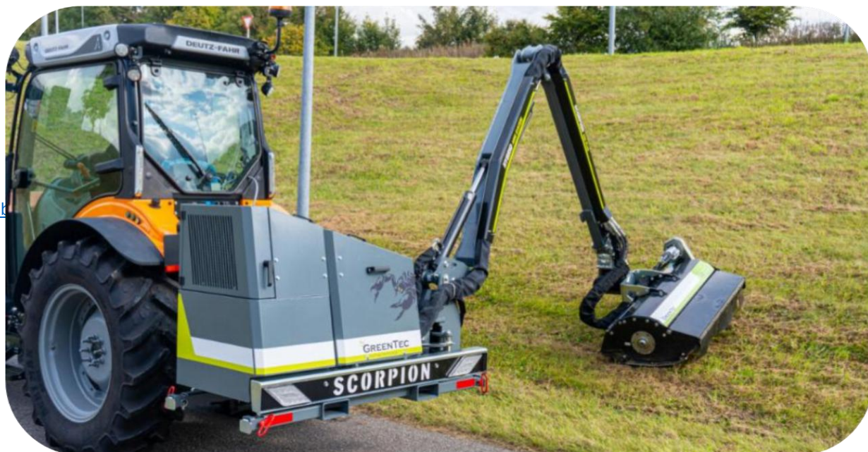
GreenTec Scorpion 490 boom mower: rear-mounted on compact tractor
