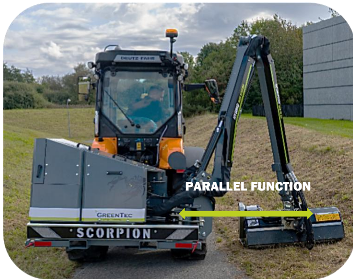
Scorpion 490 boom mower in use with parallel-functioning activated
