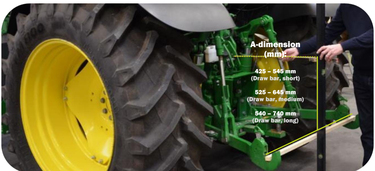
Measuring the "A dimension" on the vehicle when mounting with the upper 4-point linkage attachment on the boom mower
