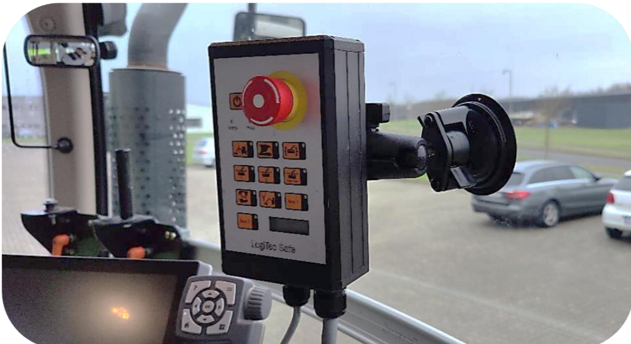
Control panel mounted up in the cabin of a vehicle using Ram-mount
