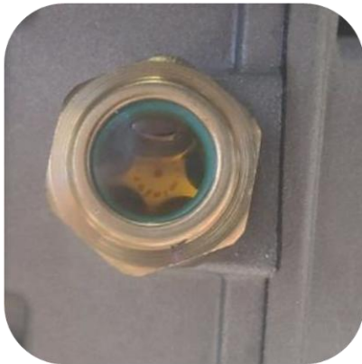
Sight glass for checking gear oil level on the gearbox
