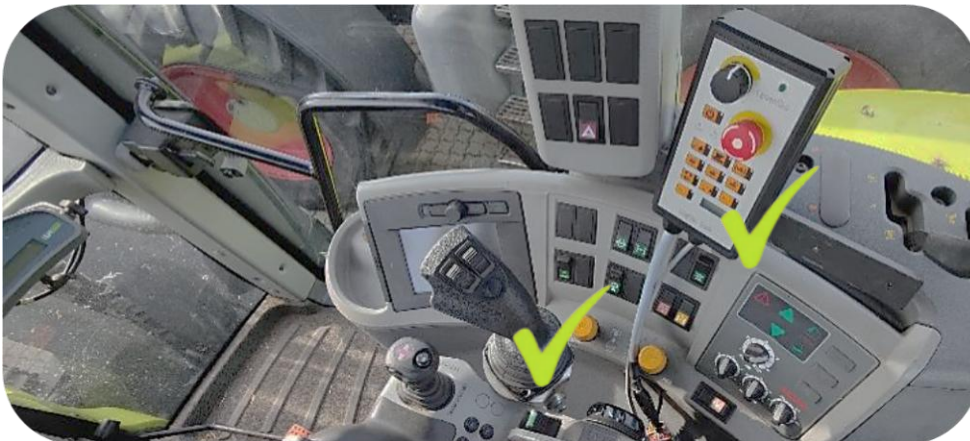
Control panel and joystick mounted and installed in cabin of vehicle
