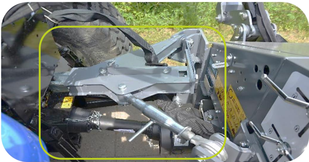
4-point mounting using 4-point linkage system with top bar attachment
