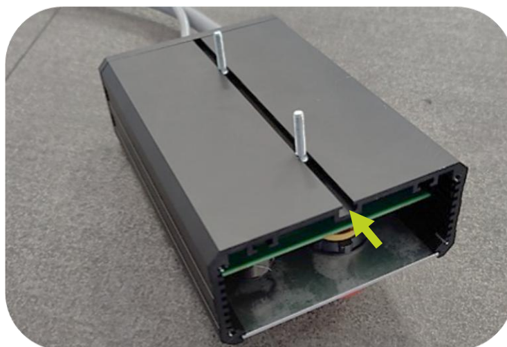
Cutout for steel set screws on the back of the control panel
