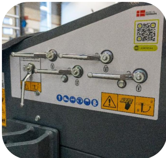
Location of transport locks / stop valves on Scorpion 490 boom mower
