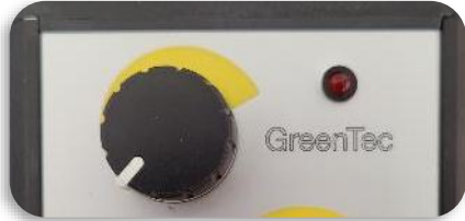
AHC potentiometer on control panel in "0" position
