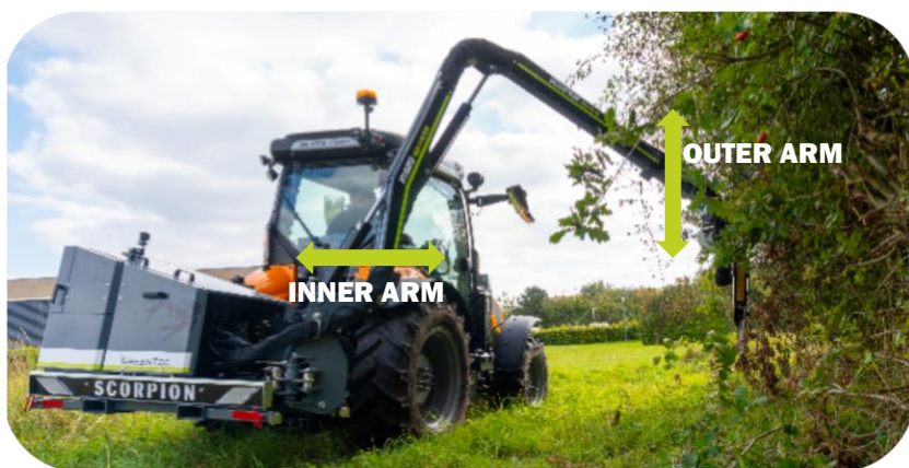
Scorpion 490 boom mower in use with non parallel-functioning activated
