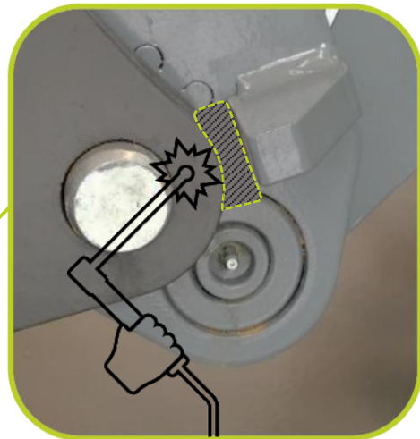
Welding on stop block
