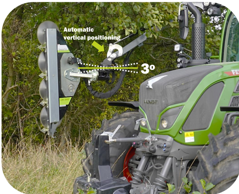
Driving with the AutoFlex-function (Automatic vertical positioning) activated: Scorpion boom mower
