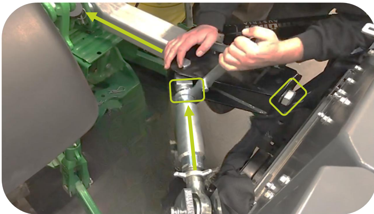
The two adjustable top draw bars are tightened/made as long as possible
